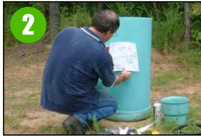
2 Determine desired location of Add-a-Branch. Use the provided adhesive template to mark location.
