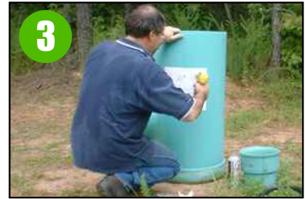
3 Use 1/2" drill bit to drill a saw starter hole at the location marked on the template.
