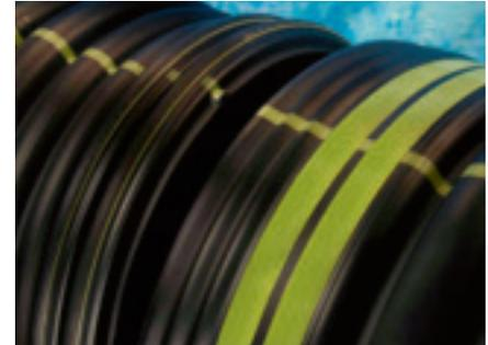
Multiple ceramic/polymer wraps are used on the longer bell to provide additional sealing area and ease of field joint assembly. The spigot has been designed with space for a second optional gasket to provide redundant sealing of the joint. These modifications provide a water-tight yet flexible joint tailored for the low head irrigation market.
